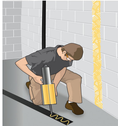
Step 2: Mix & Apply StrongHold™ Resin Wall and Carbon Strap
