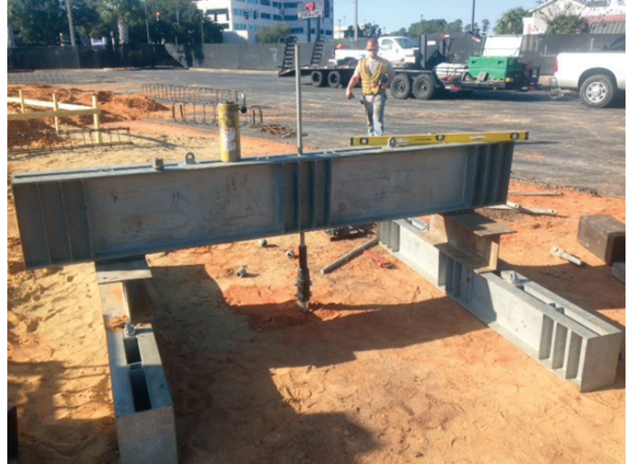
Load test conducted on a RS875.203 Pipe Pile
