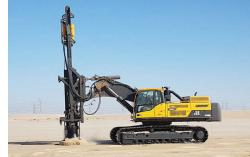
**RIC (Rapid Impact Compaction)** Use your excavator for ground compaction work. Fast, economical and dynamic ground compaction technique for low cost ground improvement of non cohesive soils.
