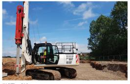
JX Piling RIG Introducing the all new BSP JX25 piling rig based on a 20 tonne excavator. Designed for driving most types of foundation piles.
