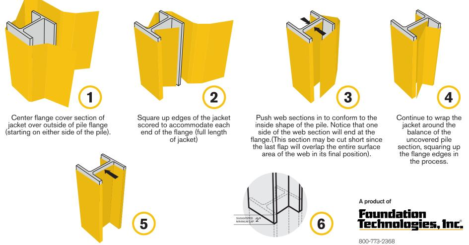
Fold the last flap back into the pile web area overlapping the previously covered web section of the pile as shown in step number 3. Flap will lock into position completing the installation.
