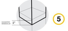
As each section is installed, lap as shown until the desired length of the pile is covered.
