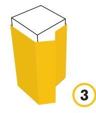
Continue to wrap jacket around balance of uncovered pile section, squaring up the scored edges at the pile corners.
