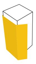
Square up edges of Jacket scored to accommodate each end of the pile corners (full length of jacket)
