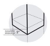
As each section is installed, lap as shown until the desired length of the pile is covered.
